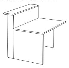
3. Screw the junction plates of the transaction module to the legs of the reception table. (3 screws per plate)
