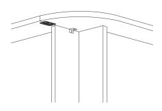
3. Install the junction plates on the insides to attach the table. (see p. 3)
