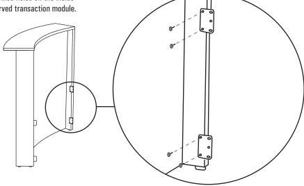
2. Attach the legs to the transaction module by screwing them to the junction plate. (3 screws per plate)
