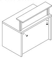
Screw from under the surface into the pre-drilled holes.
