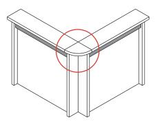
1. Place the 2 straight transaction modules at 90 degrees.
