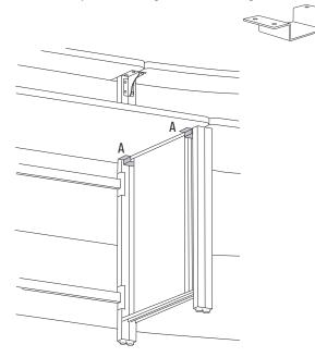
2. Install the junction plate under the shelves, when the units are placed side-by-side.
