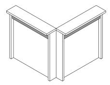
2. Attach the junction shelf to the transaction modules using the 2 L brackets and the 2 junction plates.
