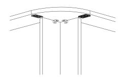
3. On the interior of the transaction module and with the metal attachment provided, attach the 2 transaction modules together at their base.
