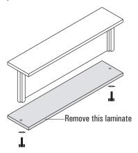
2. Place and position the shelf on the reception table in line with the pre-drilled holes on the surface.
