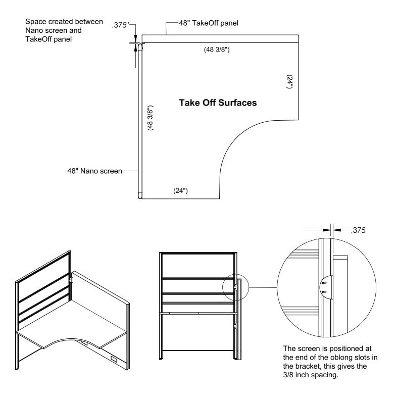
The Nano screens adapt to the TakeOff System, even when the TakeOff surfaces are 3/8" longer than Uni-T and Nano.
