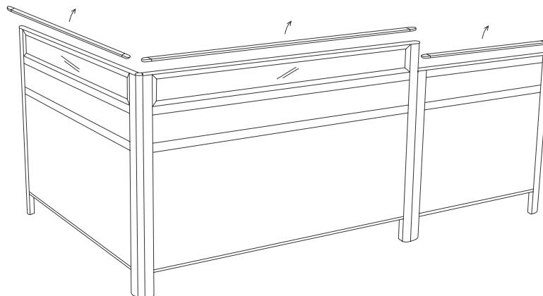
2. Insert the supports in the vertical channels of the panels and screw just until it is held lightly in place.
