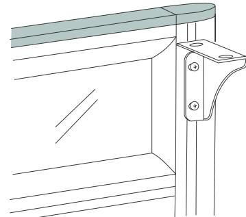
4. Move the supports until they are positioned level with the top cap and screw tightly in place.
