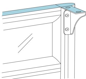
5. Place the transaction shelf on the supports and screw them together. Add junction plates if necessary.
